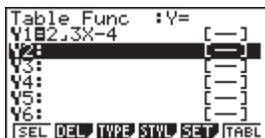
2. The default setting for tables is: X starts at 1, ends at 5, and increases by increments of 1. You change this by pressing **F5** (SET). When complete, press **EXIT**, then **F6** (TABL).
