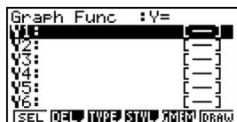
You can change the type of graph (r = polar coordinates, parametric functions, x =, and y-inequalities) by pressing **F3** (TYPE), then selecting the corresponding TYPE button. Press **▶** to begin inputting information.
