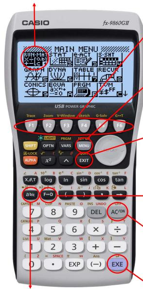
The function keys allow you to access the tab (soft key) menus that will come up at the bottom of the screen. When an appears above the key, selecting will offer more on-screen choices.
